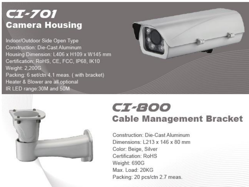
Figure 38: Camera housing and support specifications [48]
