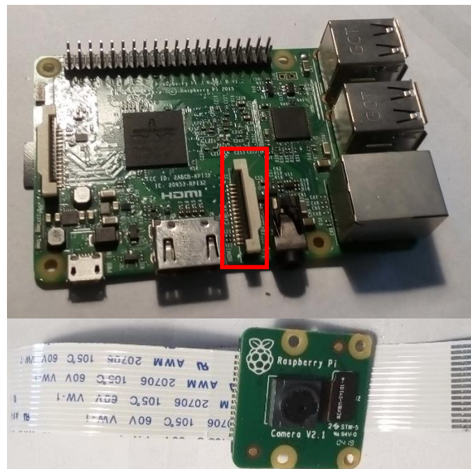
Figure 19: image sensor hardware (a) Raspberry Pi model 3B+ (Camera port highlighted) (b) V2 Pi Camera
