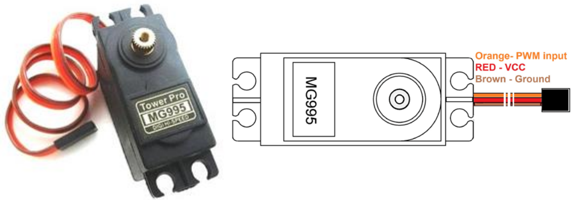
Figure 32: Servo specifications Left: Tower Pro MG995 Servo; Right: Wire color-coding [44]
