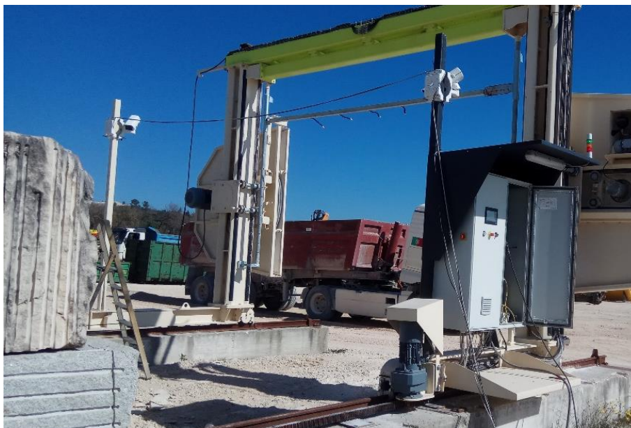
Figure 41: Scanning system installed on Fravizel cutting machine
